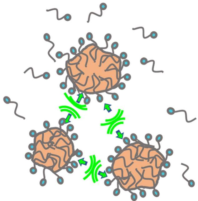
**Fig. 6** Active crystals embedded with LipiSperser<sup>®</sup> in water. Repulsive forces between the particles prevent agglomeration or aggregation, allowing LipiSperser<sup>®</sup>-coated powders to have proper particle dispersion in water
