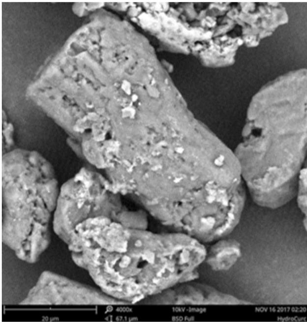
**Fig. 3** Same curcumin crystals but now coated with LipiSperser<sup>®</sup>. Crystals are less angular and much smoother in appearance. The hydrophilic heads of the surfactant molecules are on the surface and ready to interact with water. In addition, less angles and less roughness decrease the contact angle with water, which increases dispersion in water
