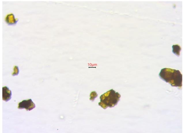
**Fig. 5** Curcumin powder coated with LipiSperser<sup>®</sup> in water. Crystals are pushing each other apart—as seen under optical microscope (AmScope) at  $\times 40$
