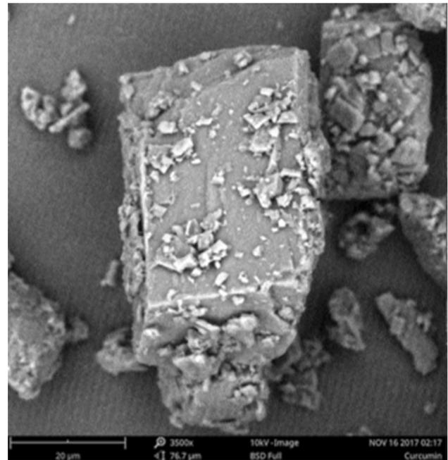
Fig. 2 Curcumin crystals viewed under scanning electron microscope (Phenom) at  $\times 3500$  magnification. Crystal structure is very chiselled and angular with a high degree of agglomeration with smaller particles and roughness. All of these factors decrease the crystal's ability to disperse in water
