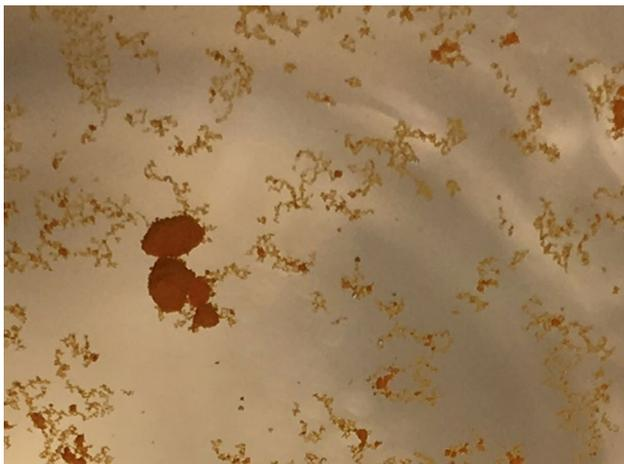
**Fig. 4** Pure curcumin powder in water. Crystals are sticking together and agglomerating
